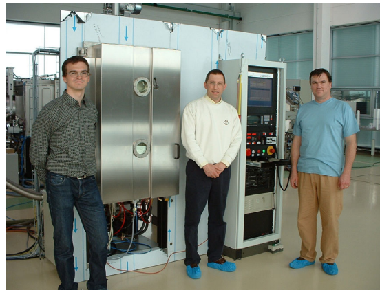
Thin film evaporator LAB 600 H (Leybold Optics) - designed for lift-off - ion assisted evaporation
