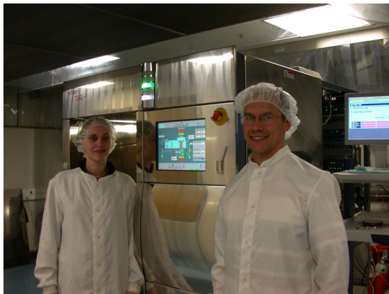
Plasma etcher (ICP) AMS 200 DSE (Alcatel) - deep SiO 2 etching (>20um) - SOI etching without notching - electrostatic chuck
