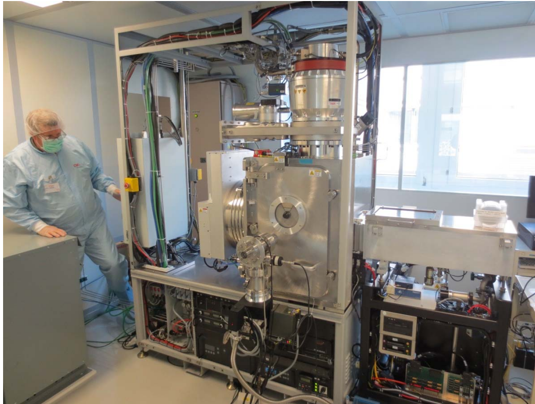
Veeco IBE NEXUS IBE350Si (Installed in 2013)
